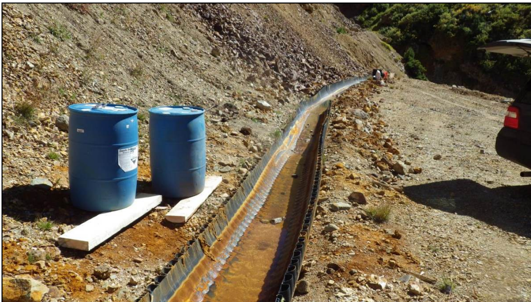
Figure 24.—Photograph showing seepage flow in the half-pipe channel at the Gold King Mine Level 7 New Adit area on September 11, 2014. Flow of approximately 12.6 gpm was recorded (photograph from EPA project files).
