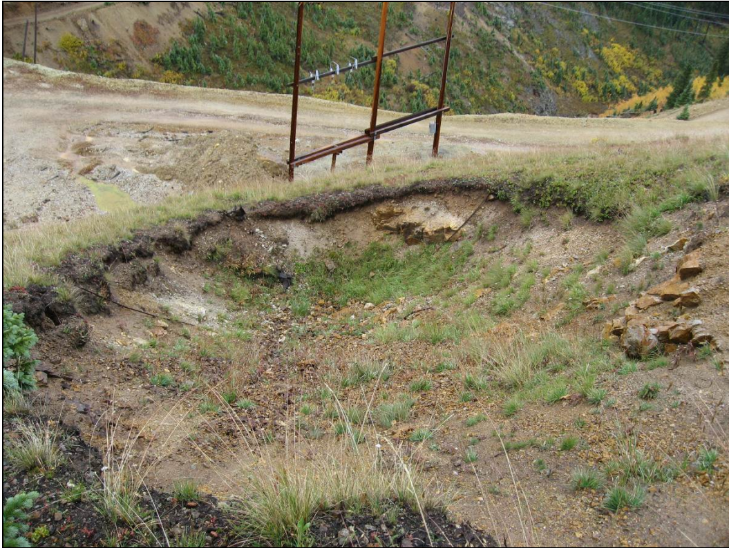
Figure 32.—Photograph taken on September 22, 2014, looking downhill at the subsidence pit located above the Gold King Mine Level 7 Old Adit.
